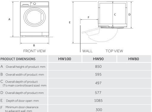
Note: The exact height of your washer is dependent on how far the feet are extended from the base of the machine. The space where you install your washer needs to be at least 40mm wider and 20mm deeper than its dimensions.
